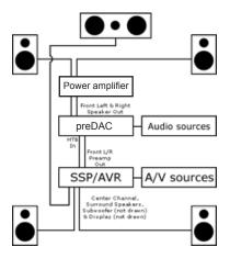
Connect Line-level (RCA style) front left and right outputs from the SSP or AVR to the **AUX-1/HTB** input on the preDAC.
